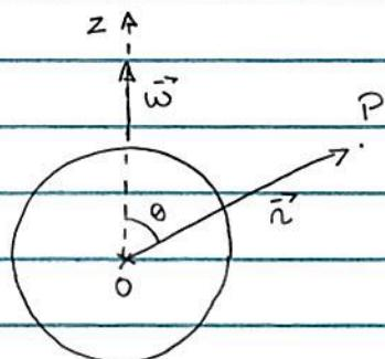
$$\hookrightarrow \vec{\kappa}(\vec{n}) = \vec{\kappa}(n, \theta) = \sigma \vec{v} = \sigma (\vec{\omega} \times \vec{n}) = \sigma \omega n \sin \theta \hat{\phi}$$
