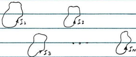
$$\hookrightarrow \phi_i = \phi_{ii} + \phi_{i2} + \dots + \phi_{ii} + \dots + \phi_{in} = \sum_{j=1}^n \phi_{ij} : \text{Fluxo total através circuito } \Gamma_i$$
