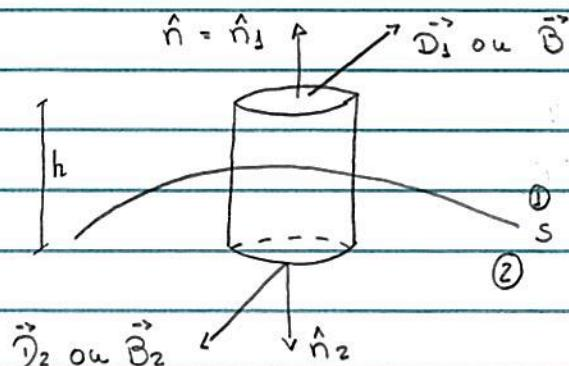
$$\text{Eq. (243.1)} : \oint_{\text{CILINDRO}} \vec{D} \cdot d\vec{s} \xrightarrow{h \rightarrow 0} (\hat{n}_1 \cdot \vec{D}_1 + \hat{n}_2 \cdot \vec{D}_2) A = Q_f = \sigma_f A$$
