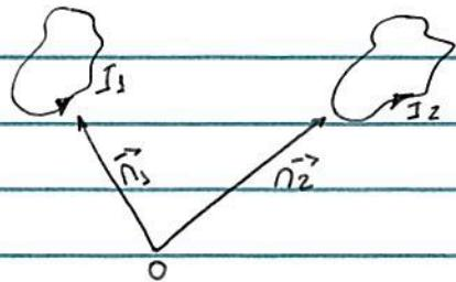
$$\hookrightarrow \phi_{21} = \int_{S_2} \vec{B}_1 \cdot d\vec{s} = \int_{S_2} (\vec{j} \times \vec{A}_1) \cdot d\vec{s} = \oint_{\Gamma_2} \vec{A}_1(\vec{n}_2) \cdot d\vec{e}_2$$
