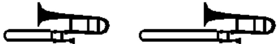
The natural frequency of a trombone can be modified by changing the length of the air column inside the metal tube.
