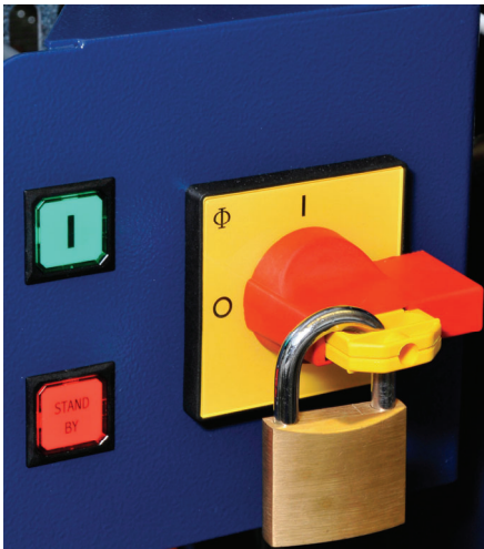
Fig. 9: System can be secured against unauthorized use by safety lock. Switch On of system is impossible when locked. All internal lines other than those marked by orange isolation are cut from electrical power supply. Generation of X-rays is impossible when system is locked.
