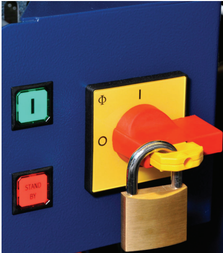
Fig. 13: System can be secured against unauthorized use by safety lock. Switch On of system is impossible when locked. All internal lines besides those marked by orange isolation are cut from electrical power supply. Generation of X-rays is impossible when system is locked.
