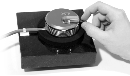
Figure 3-7: Placing the Sample Holder in the Scan Head
