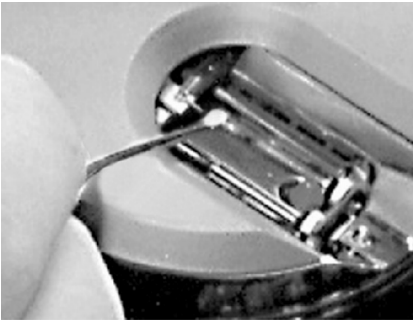
Figure 8-2: Cleaning the sample holder guide bars
