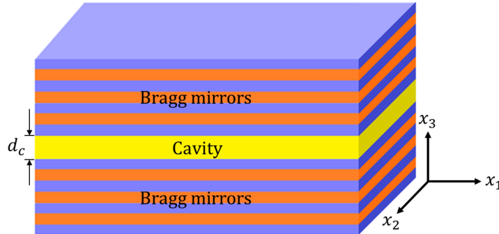
Figure 3.9: illustration of a POMC. The cavity layer, represented in yellow, is inserted between two BMs.
