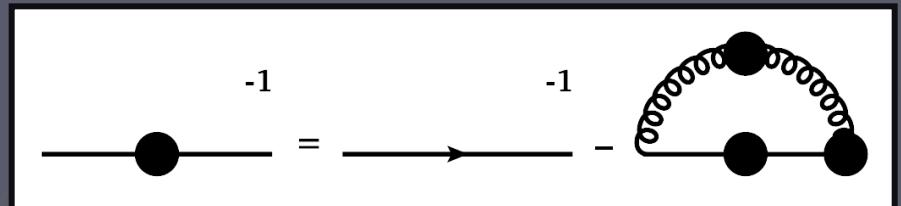
$$S_B^{-1}(p, \Lambda) = S_0^{-1}(p) + \int d^4q g_B^2(\Lambda) D_{\mu\nu}^B(p - q, \Lambda) \frac{\lambda^a}{2} \gamma_\mu S_B(q; \Lambda) \Gamma_{B\nu}^a(q, p; \Lambda)$$
