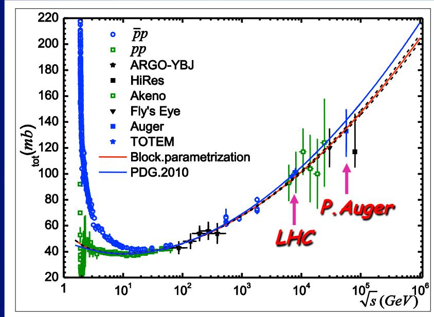
$$\sigma_{\text{PDG}}^\mp(s) = a_0 + a_1 A_1^{b_1} \mp a_2 A_1^{b_2} + a_3 \ln^{b_3}(A_2)$$
