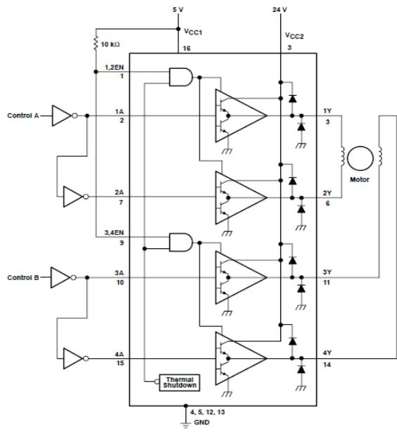
Figure 3. Two-Phase Motor Driver (L293D)
