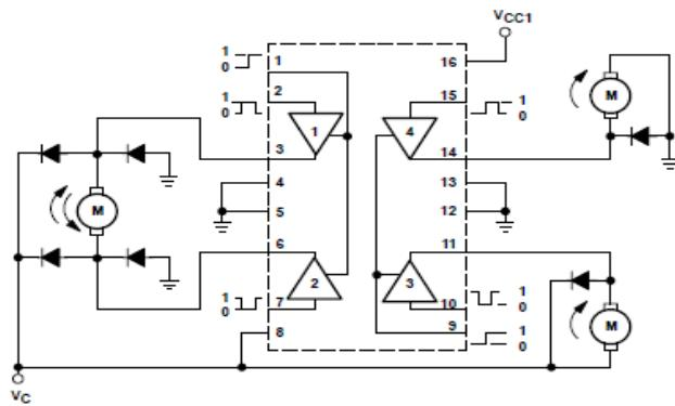
NOTE: Output diodes are internal in L293D.
