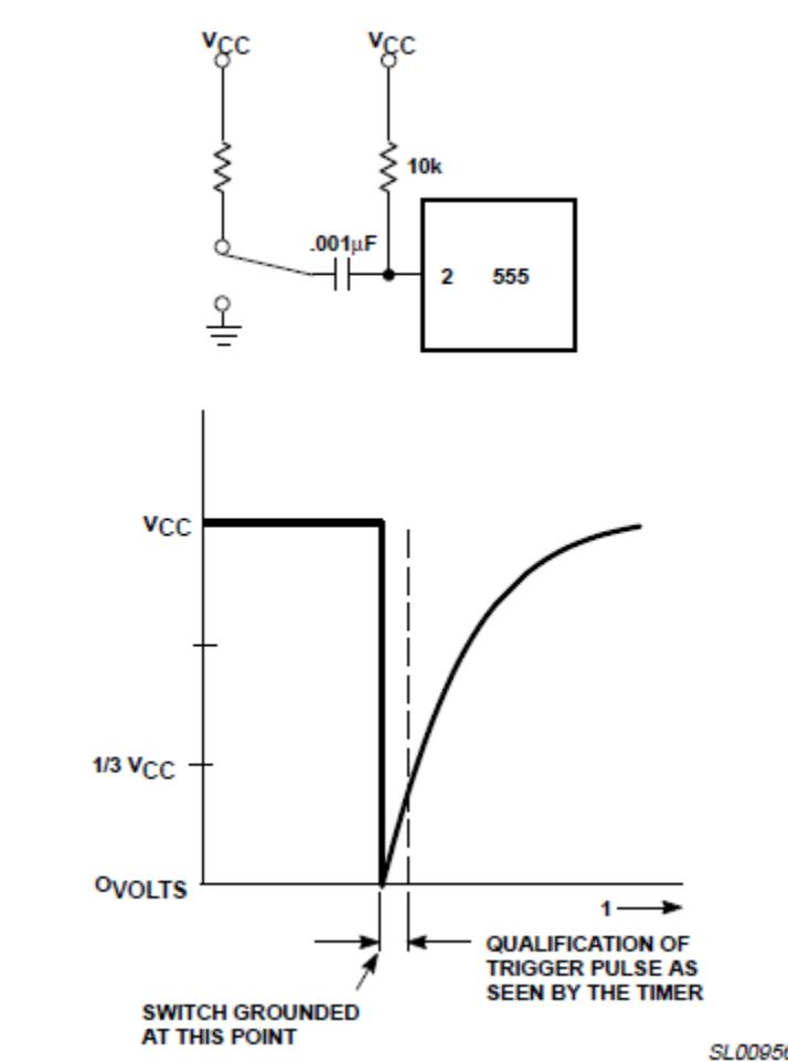
*Upon application of the negative pulse to pin 2, the FF is Set which releases de schort circuit across the external capacitor C and drives the output High. The capacitor charges in a time  $1.1R_A C$ . When the voltage across the capacitor reaches  $2/3 VCC$ , the comparator resets the FF discharging C and output goes Low.*
