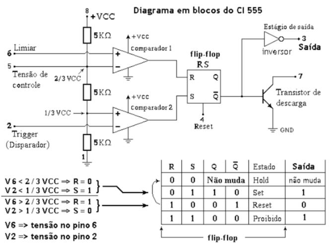
The 555 timer consists of two voltage comparators (op amplifiers), a bistable flip-flop, a discharge transistor, and a resistor divider network. See the block form in Figure. A Monostable circuit.
