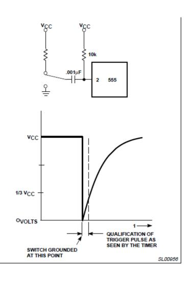
Uppon aplication of the negative pulse to pin 2, the FF is Set which releases de schort circuit across the external capacitor C and drives the output High. The capacitor charges in a time  $1.1R_A$  C. When the voltage across the capacitor reaches 2/3 VCC, the comparator resets the FF discharging C and output goes Low.
