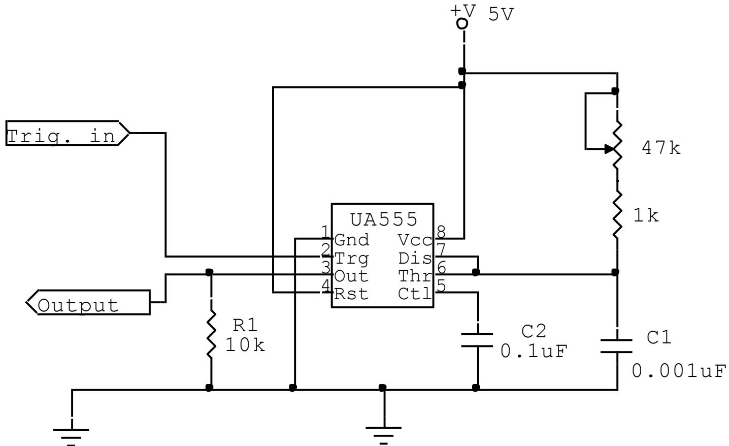
**By AC coupling the trigger , a short negative-going pulse is achieved when the trigger signal goes to ground.**
