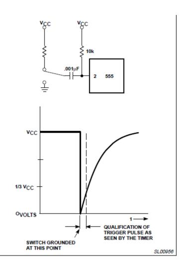
Uppon aplication of the negative pulse to pin 2, the FF is Set which releases de schort circuit across the external capacitor C and drives the output High. The capacitor charges in a time  $1.1R_A$  C. When the voltage across the capacitor reaches 2/3 VCC, the comparator resets the FF discharging C and output goes Low.
