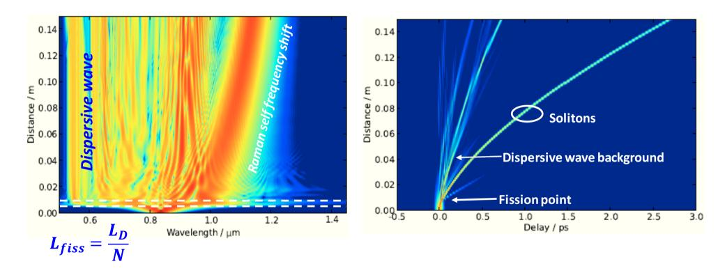
Alternatively – use normally dispersive fibre and SPM
