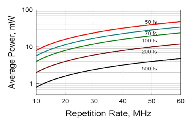
At repetition rates from a conventional fibre laser, for pulse durations in the 500fs-1ps regime only a few mw average power is required
